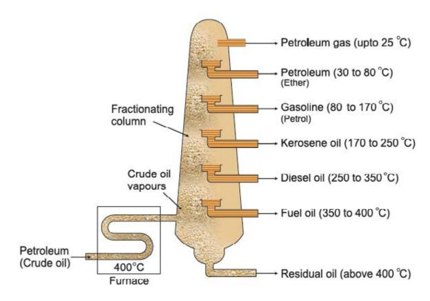
Fig 16.11 Fractional distillation of petroleum.
