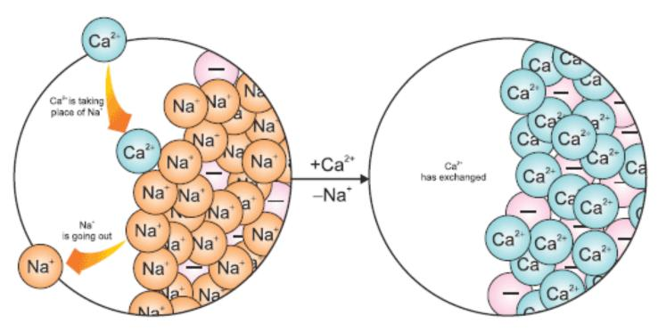
Fig. 15.3 Ion exchange for removal of hard water ions
