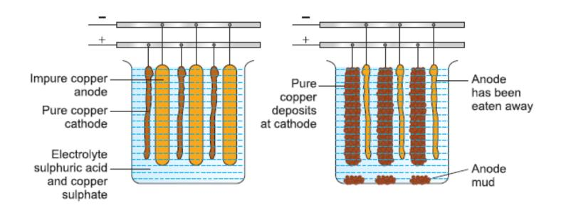
Fig. 16.6 Electrorefining of copper.
