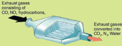
Fig.14.5: Catalytic Converter Used in automobile vehicles.
