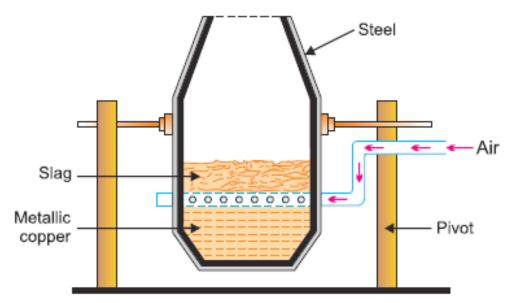
Fig. 16.5 Bessemer converter used for bessemerization of copper.
