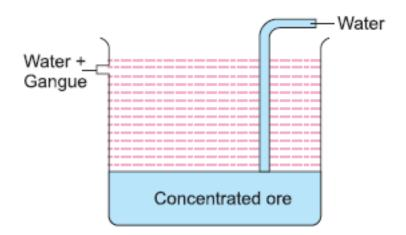
Fig. 16.1 Gravity separation
