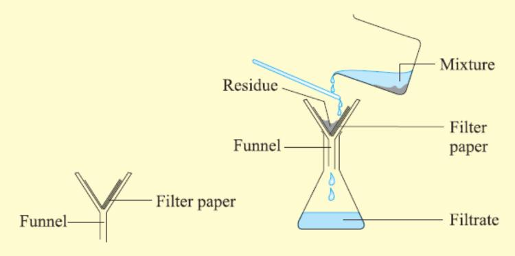
Filtrate passes through the filter paper and is collected in a conical flask. The solid particles (residue) deposit on the filter paper. It is then dried.
