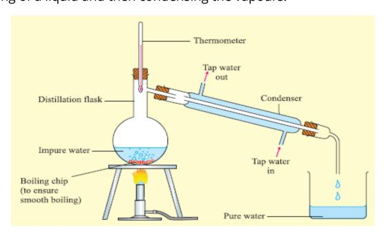
Impure water is taken in a distillation flask. It is boiled. Water vapours rise and enter the condenser. The vapours condense while passing through condenser. Thus, they are changed back into pure water, which is called distillate (distilled water). The distillate is collected in a beaker. The impurities remain behind in the distillation flask.
