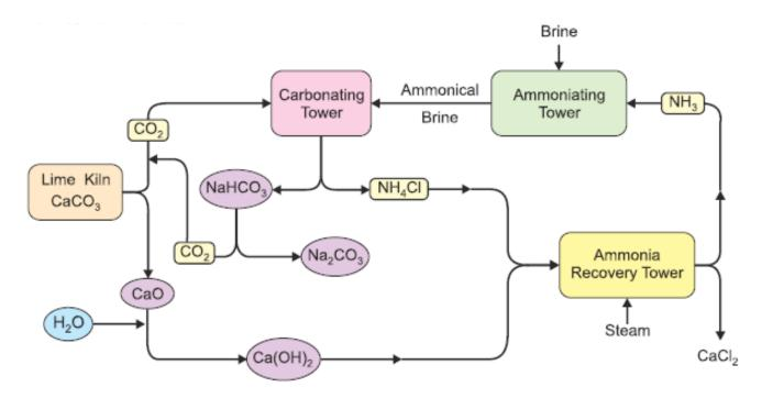
Fig. 16.8: Flow sheet diagram of Solvay's Process for the manufacturing of sodium carbonate.
