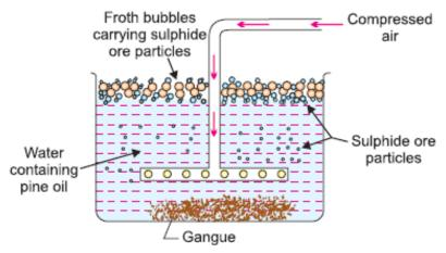
Fig. 16.2 Froth flotation process
