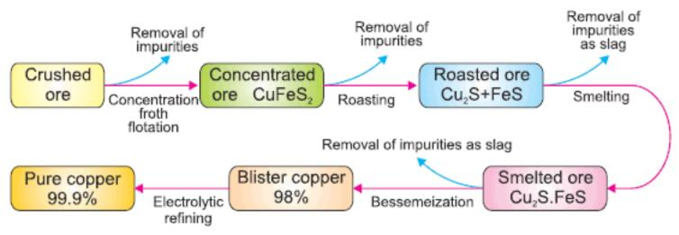
Fig. 16.7 Flow sheet diagram for extraction of copper
