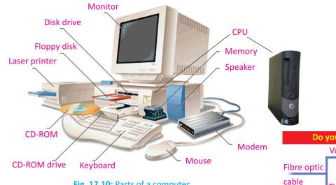
Fig. 17.10: Parts of a computer
