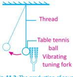
**Fig. 11.3:** The production of sound waves from a vibrating tuning fork
