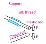
**Fig.13.2:** Two plastic rods rubbed with fur repel each other
