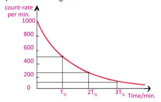
Fig. 18.8: Decay of unstable element
