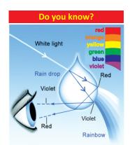
Dispersion of light is due to the variation in refractive index with the colour. Dispersion in drops of water separates the colours of sunlight into a rainbow.
