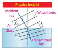
In refraction, the speed of light changes due to change in the wavelength. But, frequency and hence the colour of light does not change.
