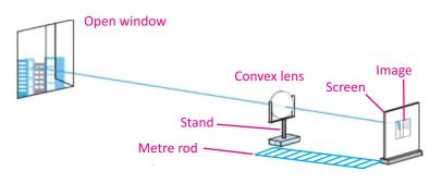
Fig.12.22: Approximate method of finding focal length of a convex lens
