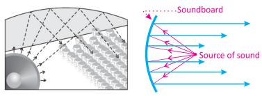
Fig. 11.11: Curved ceiling of a conference hall Fig. 11.12: Soundboard used in a big hall 11.7 AUDIBLE FREQUENCY RANGE
