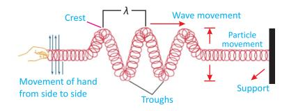
Fig. 10.9: Transverse wave on a slinky
