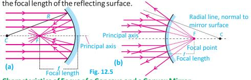
Characteristics of Focus of a Concave and a Convex Mirror
