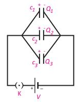
Fig.13.14: Capacitors in parallel combination
