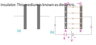
Fig. 13.13 (a) Parallel plate capacitor (b) Plates of capacitor connected with battery
