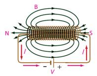
Fig. 15.4: Magnetic field due to a solenoid
