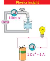
The flow of charge in a circuit is like the flow of water in a pipe except that a return wire is needed in order to have a complete conducting path.
