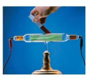
A cathode ray will deflect as shown when it is under the influence of an external magnetic field.
