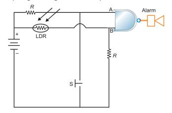
Fig. 16.16: Burglar alarm schematic circuit
