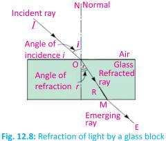
At the air-glass interface, the ray of light IO changes direction and bends towards the normal and travels along the path OR inside the glass block. The rays IO and OR are called the incident ray and the refracted ray respectively. The angle *'i'* made by the incident
