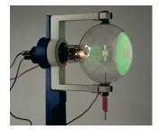
In a cathode-rays tube, a greenish glow is formed on the inner surface of the glass opposite the cathode, which itself is glowing orange here. The shadow cast by the cross at the centre of the tube gives evidence that rays of some kind are passing through the tube.
