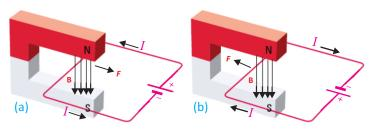
Fig. 15.6: Force on a current-carrying wire in magnetic field
