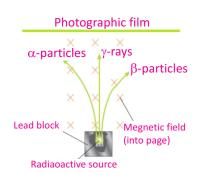
**Fig.18.3:** Three types of radiations can be distinguished from their path followed in an external magnetic field
