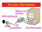
By using an oscilloscope, you can "see" sound waves.
