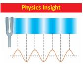
Illustration of longitudinal wave formed by vibrating tuning fork in the air. Compressions are places where air pressure is slightly higher than the surrounding air pressure due to high density of air particles. While rarefactions are the regions correspond to low air pressure due to low density of air particles.
