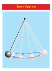
Time period of a pendulum is the time to complete one cycle.
