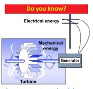
A generator inside a hydroelectric dam uses electromagnetic induction to convert mechanical energy of a spinning turbine into electrical energy.
