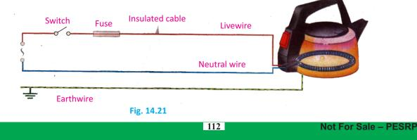
However, the earth terminal is connected to the metal casing, so the current goes through the Earthwire instead of passing through our body and causing an electric shock. A strong current passes through the Earthwire because it has a very low resistance. This breaks the fuse and disconnects the appliance.
