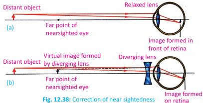
The nearsighted eye can be corrected with glass or contact lenses that use diverging lenses. Light rays from the distant objects are now diverged by this lens before entering the eye. To the observer, these light rays appear to come from far point and are therefore focused on the retina, thus forming a sharp image (Fig.12.38-b).
