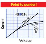
The current versus voltage graph of a resistor is a straight line with a constant slope. The graph for light bulb is curved with a decreasing slope. What can you infer from this?
