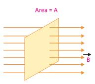
**Fig.15.10:** Maximum strength of magnetic field
