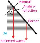
**Fig. 10.13:** Reflection of water waves from a plane barrier
