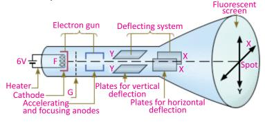
Fig. 16.4: Cathode-Ray Oscilloscope
