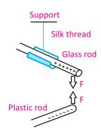
**Fig.13.3:** Plastic rod rubbed with fur and glass rod rubbed with silk attract each other
