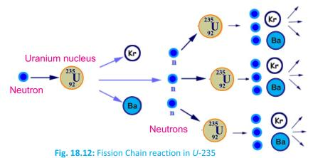
This fission chain reaction is controlled in nuclear reactors. A nuclear reactor provides energy for useful purposes. In this sort of self sustained reaction, extra neutrons liberated in fission reactions are absorbed using some material to slow down the chain reaction.
