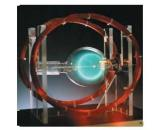
The glow in the tube is due to circular motion of electron in the magnetic field. The glow comes from the light emitted from the excitations of the gas atoms in the tube.
