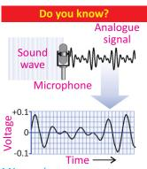
Microphone creates an analogue signal, shown by the voltage versus time graph.
