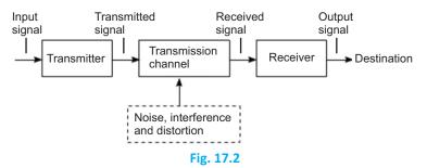
The transmitter processes the input signal. The transmission channel is the medium which sends the signal from source to destination. It may be a pair of wires, a coaxial cable, a radiowave or optical fibre cable. So, the signal power progressively decreases with increasing distance. The receiver takes the output signal from the transmission channel and delivers it to the transducer after processing it. The receiver may amplify the input signal to compensate for transmission loss.
