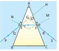
**Fig.12.17:** Refraction through a triangular glass prism
