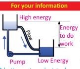
A battery raises electric charge back up to higher voltage (energy) just like a pump which pushes water back up to high energy so it can flow and do work again.
