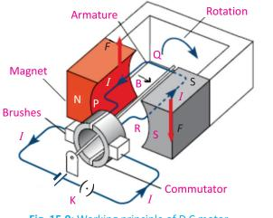
Fig. 15.9: Working principle of D.C motor
