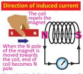
**Fig.15.15 (a)** Direction of induced current when magnet is moved towards the coil
