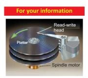
In computer hard drive, each platter has a magnetizable coating on each side. The spindle motor turns the platters at several thousand resolutions per minute (rpm). There is one read-write head on each surface of each platter.
