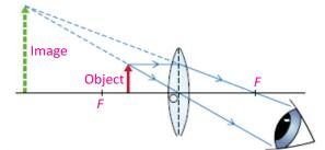
The image is behind the object, virtual, erect, larger than the object. Fig. 12.25
