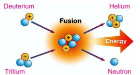
Energy coming from the Sun and stars is supposed to be the result of fusion of hydrogen nuclei into Helium nucleus with release of energy. The temperature at the centre of the Sun is nearly 20 million kelvin which makes the fusion favourable. According to this reaction, four hydrogen nuclei fuse together to form a helium nucleus alongwith 25.7 MeV of energy.
