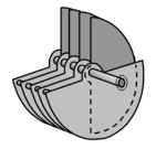
Fig. 13.19: Variable capacitor
