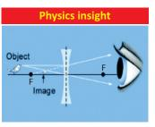
A diverging lens always has the same ray diagram, which forms a smaller image.
