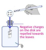
Fig.13.9 (c) Detecting negative charge on body
