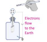
Fig.13.8 (b) Charging the electroscope positively
