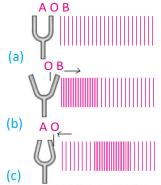
**Fig.11.6:** Vibrations of tuning fork after striking with a rubber
