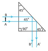
**Fig.12.10:** Total internal reflection through right angled prism
