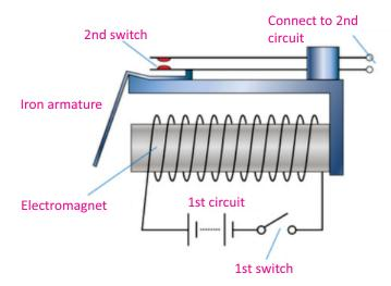
Fig. 15.21: Relay circuit
