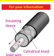
Coaxial cable wires are used to transmit electric signals such as cable TV to our homes. To prevent electric and magnetic interference from outside, a covering of conducting material surrounds the coaxial wires.
