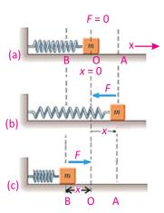
**Fig.10.1:** SHM of a mass-spring system
