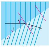
Fig. 10.15: Refraction of water waves
