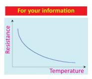
A thermister is a temperature dependent resistor and its resistance decreases as temperature rises. Thermister is used in a circuit that senses temperature change.
