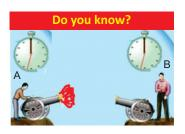
The speed of sound in air was first accurately measured in 1738 by members of the French Academy. Two cannons were set up on two hills approximately 29 km apart. By measuring the time interval between the flash of a cannon and the "boom", the speed of sound was calculated. Two cannons were fired alternatively to minimize errors due to the wind and to delayed reactions in the observers. From their observations, they deduced that sound travels at about 336 m s<sup>-1</sup> at  $0^{\circ}$ C.
