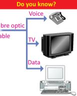
A single fibreoptic cable can carry more than enough information to support television, telephone, and computer data.
