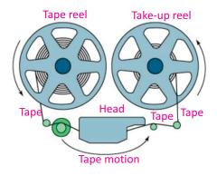
Fig. 17.13: A magnetic tape storage mechanism
