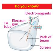
Electromagnets are used to deflect electrons to desired positions on the screen of a television tube.
