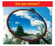
Convex mirrors produce images that are smaller than objects. This increases the view for the observer.
