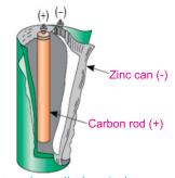
In a dry cell chemical energy changes into electric energy.
