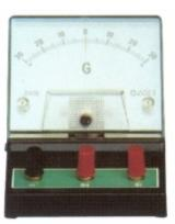
Fig.14.3: A galvanometer
