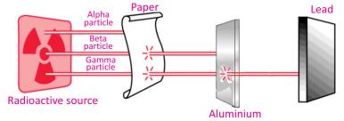
Fig.18.6: Penetrating power of radiations in different materials
