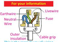
This is the correct way of wiring of a three pin main plug. Put everything in proper place. Fuse is placed for safety purpose. In case of excess current, it will burn out and will break the circuit.
