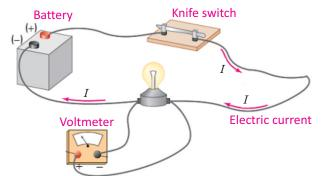
Fig. 14.8: Schematic diagram for measuring potential difference in a circuit
