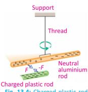
**Fig. 13.4:** Charged plastic rod attracts neutral aluminium rod.
