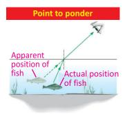
Why the position of fish inside the water seems to be at less depth than that of its actual position?
