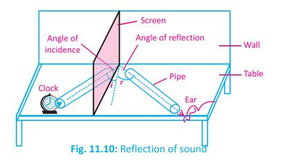
Lift the pipe on the right vertically to a small height
