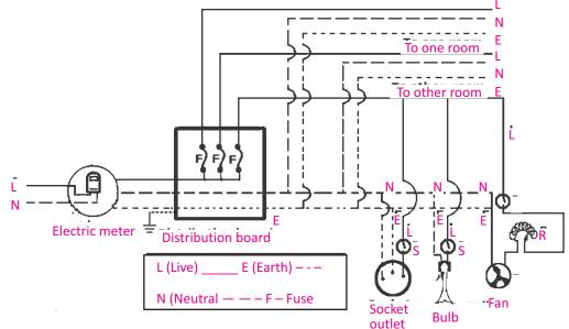
Fig.14.16: Wiring system of household electricity
