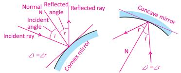
Fig.12.6: Reflection of light by spherical mirrors
