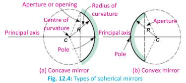
**Concave Mirror:** A spherical mirror whose inner curved surface is reflecting is called concave mirror. In concave mirror the size of the image depends on the position of the object. Both virtual and real images can be formed by a concave mirror.
