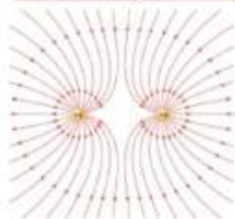
Fig.9.7: The electric field lines for two identical opposite point charges.
