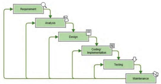
Figure 1.1: System development life cycle stages
