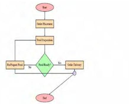
Figure 1.12: Activity Diagram with Decision and Connector Symbol
